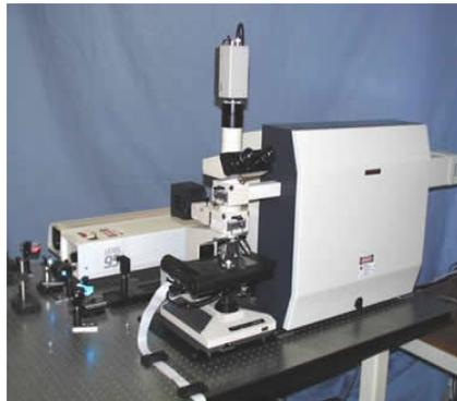
Renishaw 2000 Confocal Raman Microprobe (共焦点ラマン顕微鏡)
